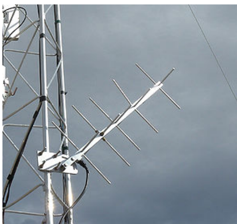
Fig. A typical circular-polarized GOES antenna for one-way burst transmission of limited data
