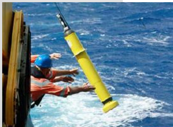
▲ The deployment of an Argo float into the ocean. Credit: CSIRO.
